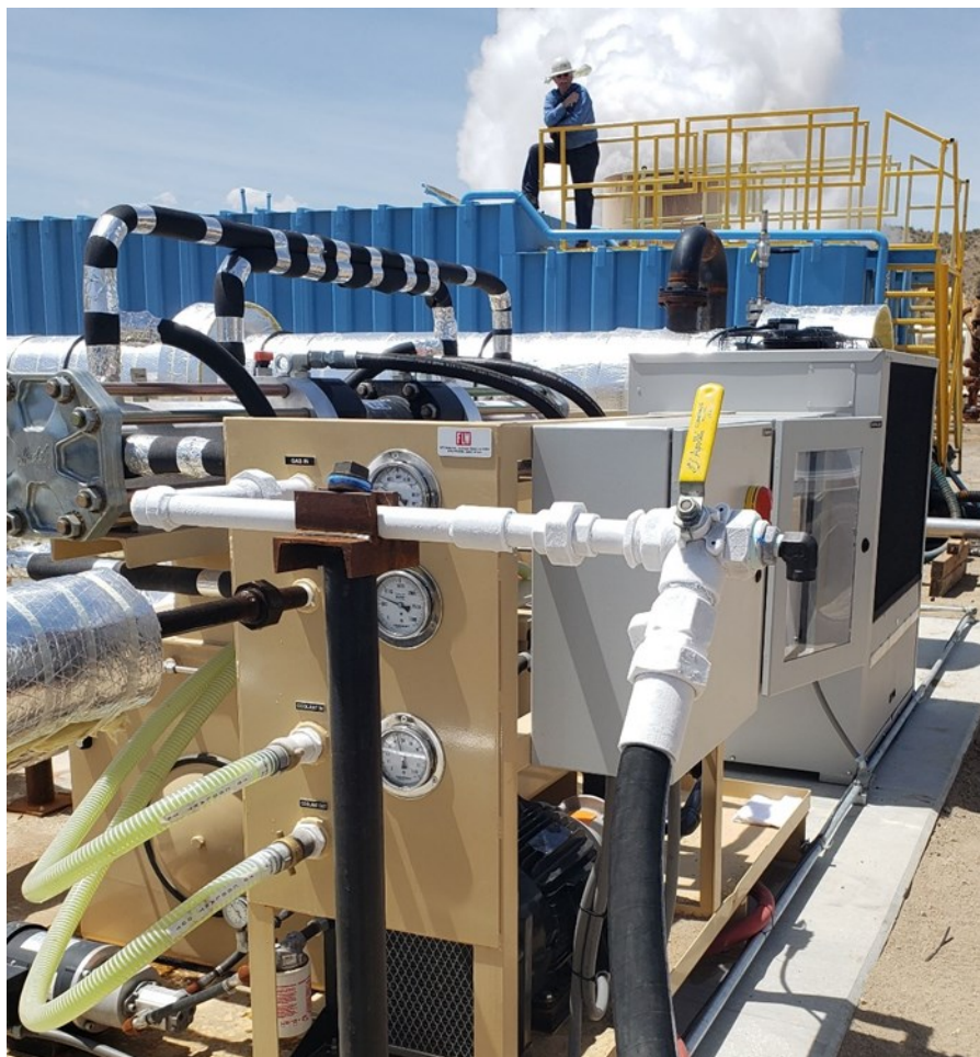
Figure 4: Photo of the demonstration equipment just after the well was opened with CO 2 being pumped into the closed-loop system.
