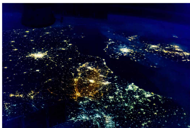
Fig. 3. Belgium and surrounding countries at night. Color-enhanced ISS image (iss038e014887, 10-12-2013). Belgium in the middle with orange color, characteristic of use of low-pressure sodium lights and with roads lit. The Netherlands, France, and the United Kingdom, at the right, left, and top, respectively, with yellowish color from high-pressure sodium lights. Germany at the bottom, with blueish color from fluorescent and mercury vapor lights. Figure S3 provides a reprojected version of this image, with country boundaries.
